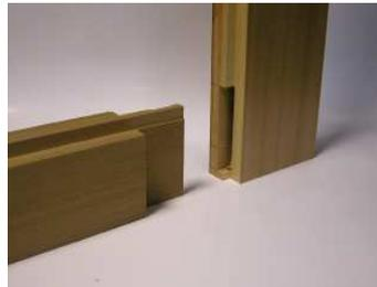
Mortice and tenon joint
